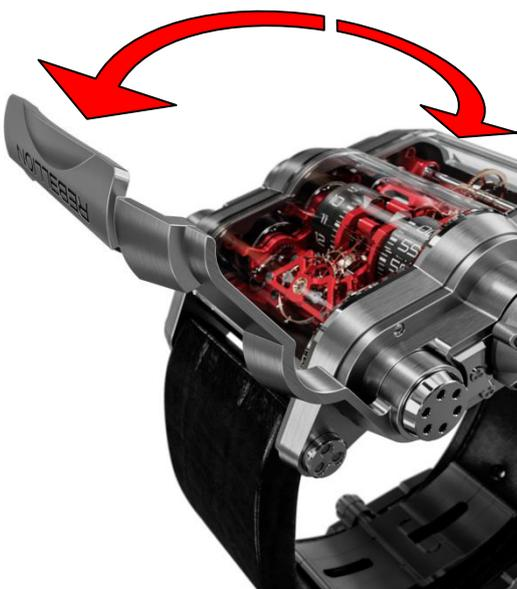
To fully wind your T-1000 watch from empty, operate the **WINDING LEVER-1** over its full span 120 times (3). **Do not force the WINDING LEVER-1** if you feel resistance, as it is an indication that the **6 mainspring barrels are fully wound**. When winding is complete, lightly press-click the **WINDING LEVER-1** back against the case. To maximize timekeeping performance, we recommend winding your T-1000 once a month.
