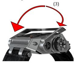
To fully wind your PROMETHEUS watch from empty, maneuver the WINDING LEVER-1 over its full span 180 times (3). Do not force the WINDING LEVER-1 if you feel resistance. That indicates that the 6 mainspring barrels are fully wound. When winding is completed, lightly press-click the WINDING LEVER-1 back against the case. То maximize timekeeping performance, we recommend winding your Prometheus once a month.
