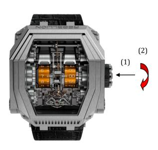
To set the time, press the PUSHER BUTTON / CULTCH-5 (1) situated in the middle of the CROWN-4 and hold it while simultaneously turning the CROWN-4 counterclockwise to adjust the hour and the minute rollers (2) to the correct time.
