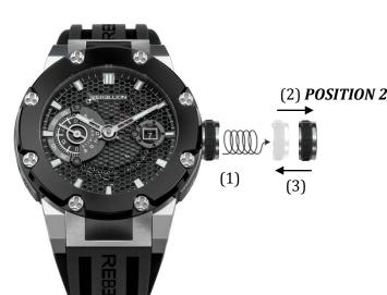
After unscrewing the crown (1), pull the crown out (2) to POSITION 2 and turn the crown clockwise to set the date. After having set the date, simultaneously push and screw the crown back to the (2) **POSITION 2** home position (details 3-7). Please never adjust the date function of your **REBELLION watch between 8pm and 3am** as it could seriously damage the movement.
