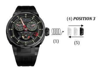
After unscrewing the crown (1), pull the crown out two clicks (4) to **POSITION 3**, adjust the hands to the correct time – clockwise (NB: around midnight the date will change), simultaneously push and screw the crown back to home position (Details 5-7). When performing this operation make sure that the calendar changes the date at midnight and not at midday. Beware: It is crucial to set time clockwise (setting time counter-clockwise can make your watch going slow).
