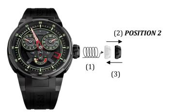
After unscrewing the crown (1), pull the crown out (2) to *POSITION 2* and turn the crown clockwise to set the date. After having set the date, simultaneously push and screw the crown back to the home position (details 3-7). Please never adjust the date function of your REBELLION watch between 8pm and 3am as it could seriously damage the movement.
