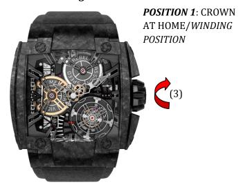
To wind your watch, in **POSITION 1**, turn the crown clockwise until the power reserve indicator shows that the watch is fully wound. Be careful not to force the winding when you feel a light resistance as it means that the watch is fully wound.
